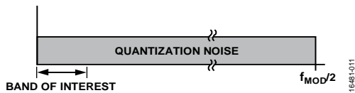
Figure 55. \Sigma - \Delta ADC Quantization Noise (Linear Scale X-Axis)
