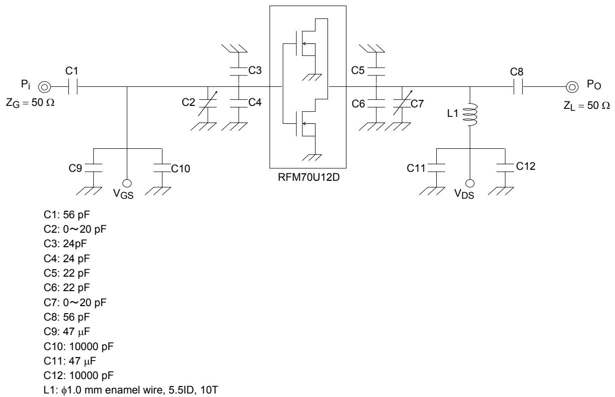
**Output Power Test Fixture**(Test Condition:  $f = 175$  MHz,  $V_{DS} = 12.5$  V,  $I_{idle} = 2$  A,  $P_i = 2$  W)
