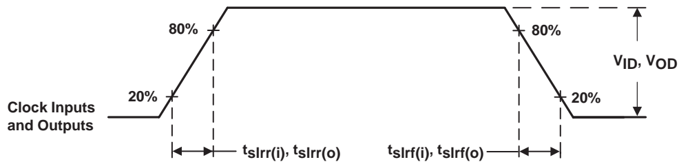
Figure 8. Input and Output Slew Rates
