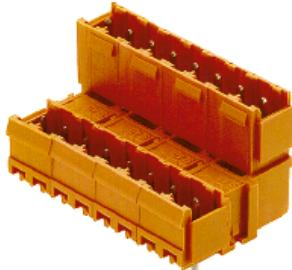
Dimensionally stable, straight, codable 2-tier male connector from the Unimate range of plugs with integral aid to prevent wrong connections. Available with open or closed sides. Fixing blocks can be attached to the closed version. The solder pin length of 3.2 mm has been optimised for wave soldering. Supplied in cardboard box.
