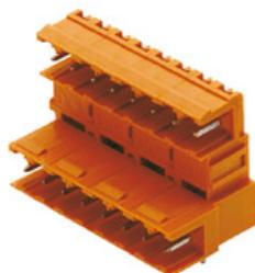
Dimensionally stable, angled, codable 2-tier male connector from the Unimate range of plugs with integral aid to prevent wrong connections. Available with open or closed sides. Fixing blocks can be attached to the closed version. The solder pin length of 3.2 mm has been optimised for wave soldering. Supplied in cardboard box.
