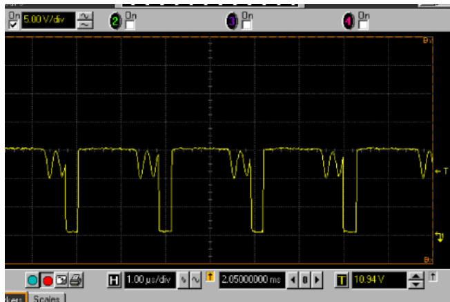
FIGURE 7. BOOST SWITCH NODE AT 100mA (PARTIAL DISCONTINUOUS)
