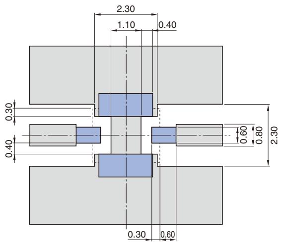
Line width be designed to match 50Ω characteristic impedance depending on PCB material and thickness.
