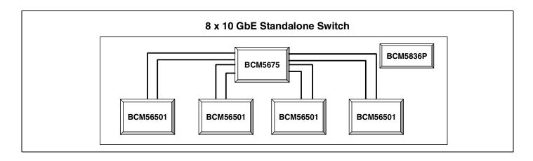
The BCM56501 is the fifth generation of the highly-integrated and costeffective StrataSwitch and StrataXGS product line. The BCM56501 is a single-chip solution with four 10-GbE/HiGig+ uplink ports.
