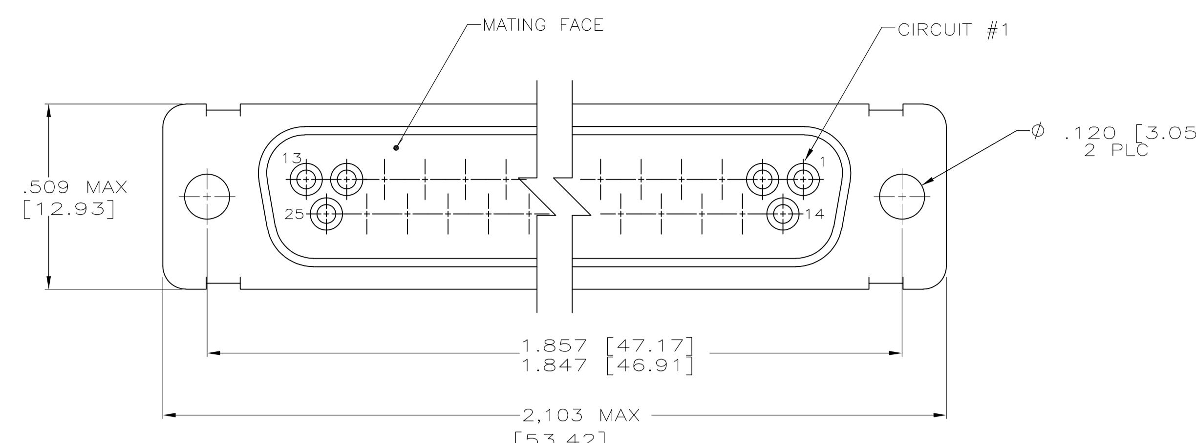
① MARKED WITH .047-.062 [1.19-1.57] HIGH CHARACTERS, FAR SIDE REFERS TO THE WIDE SIDE OF THE KEYSTONE. NEAR SIDE REFERS TO THE NARROW SIDE OF THE KEYSTONE. IF REAR SHELL IS TOO SMALL FOR AMP, AMP PART NO. REV LEVEL AND DATE CODE, THEN SPLIT AS FOLLOWS:
