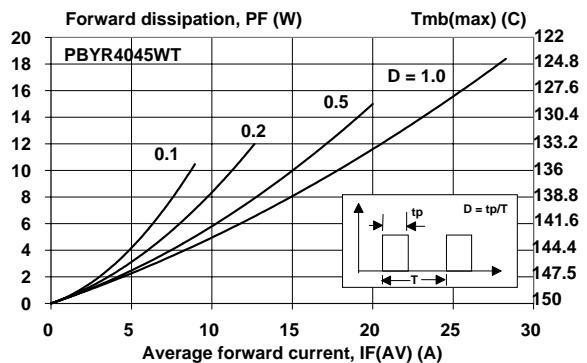
Fig.1. Maximum forward dissipation  $P_F = f(I_{F(AV)})$  per diode; square current waveform where  $I_{F(AV)} = I_{F(RMS)} \times \sqrt{D}$ .
