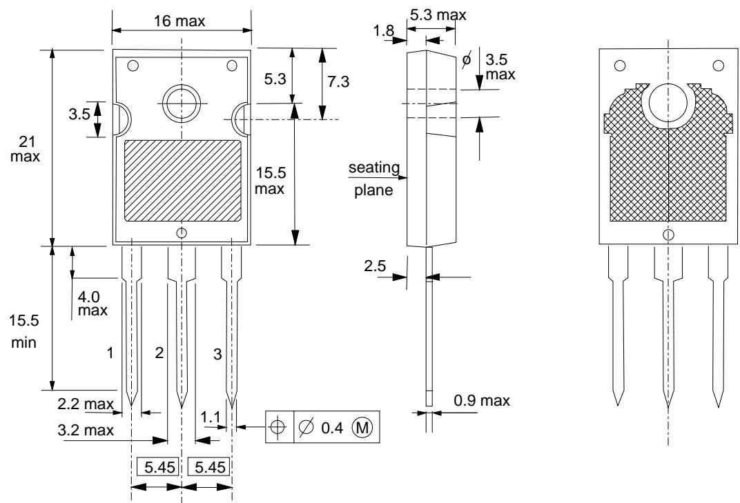
Fig.7. SOT429 (TO247); pin 2 connected to mounting base.
