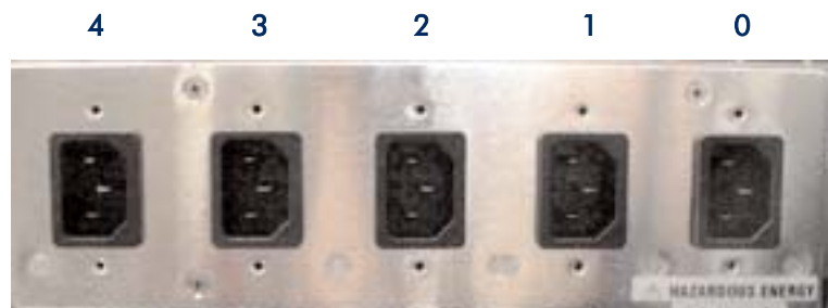
Figure 9 - Individual AC feed (IEC320/C13 shown)
