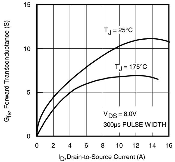
**Fig 4.** Typical Forward Transconductance vs. Drain Current
