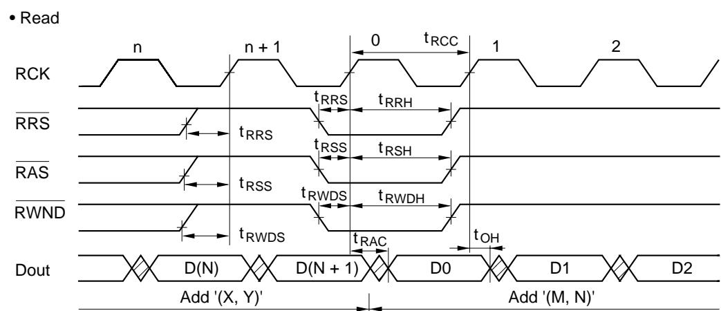
Note: The value (M, N) is the address input during the read address setup cycle.
