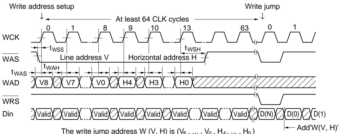
Note: The jump to the set address can be performed at any time once the required 64 cycles have passed following the start of write address setup.
