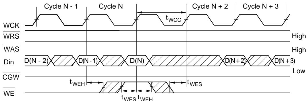
Note: Although the write address pointer is incremented on a cycle where WE is high, the  $D_{IN}$  data is not written, and the previous memory data is retained.
