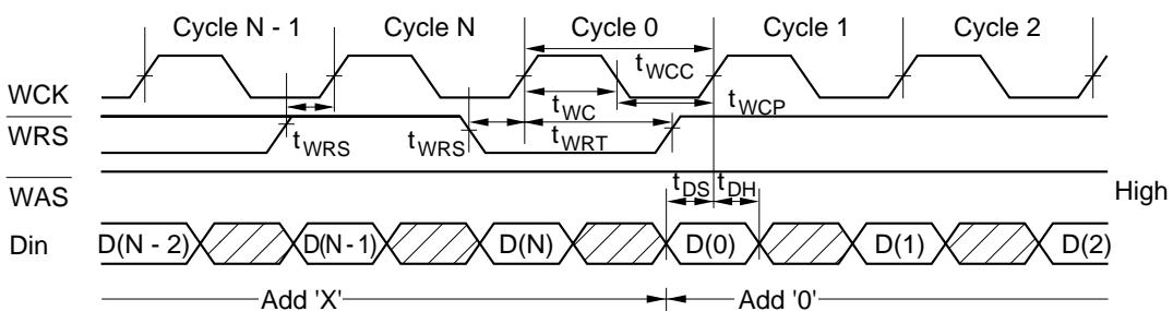
Note: The write address pointer is reset to 0 starting with the WRS low cycle. Only the falling edge of the WRS signal is detected. Adequate margin is provided if the rise occurs at least one clock cycle before the next fall.
