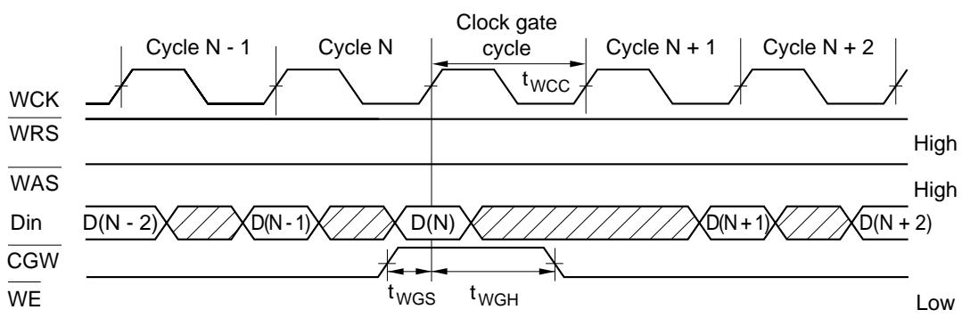
Note: During cycles where CGW is high, the write address pointer is not incremented, and the  $D_{IN}$  data is not written.
