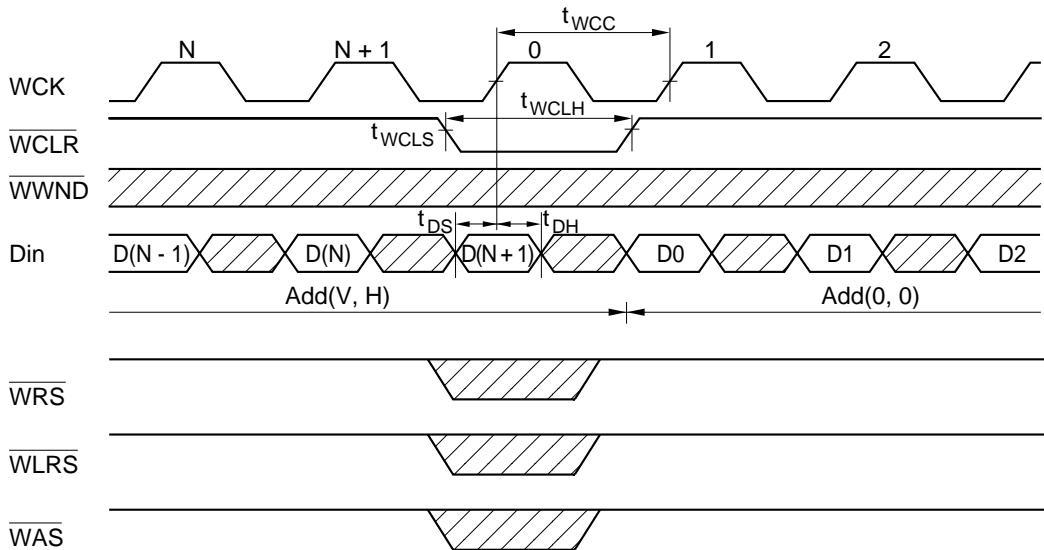
Note: The write address pointer is reset to (0, 0), and window mode is turned off if it was on.
