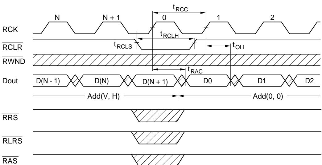
Note: The read address pointer is reset to (0, 0), and window mode is turned off if it was on.
