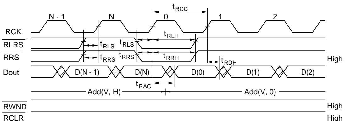
Note: The line address V is held as it is, and the horizontal address H is reset to 0.
