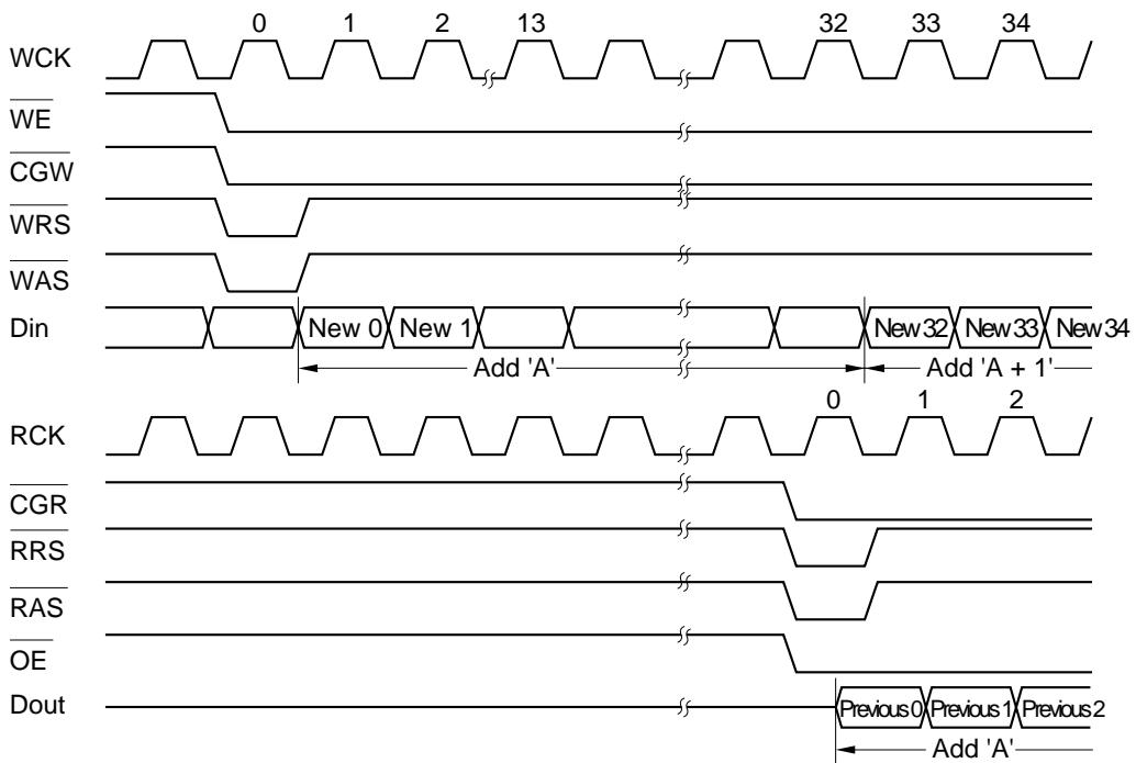
Note: Previous data can be read out up to 32 WCK clock cycles after the write operation.
