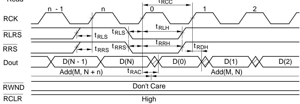
Note: The line address M is held at its current value and the horizontal address currently at  $N + n$  is reset to N.
