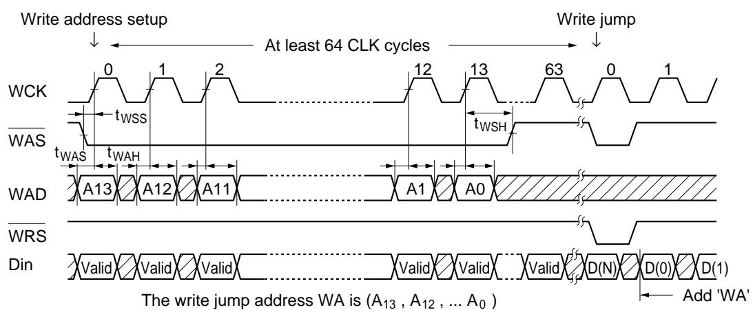
Note: After 64 cycles have passed following the start of write address setup, a jump to the set address can be performed at any time.
