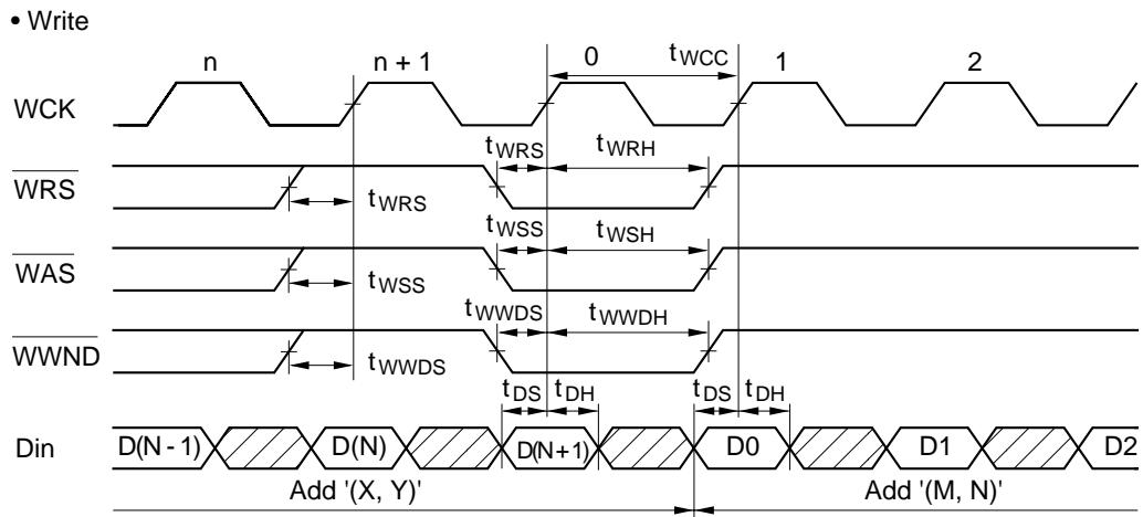
Note: The value (M, N) is the address input during the write address setup cycle.
