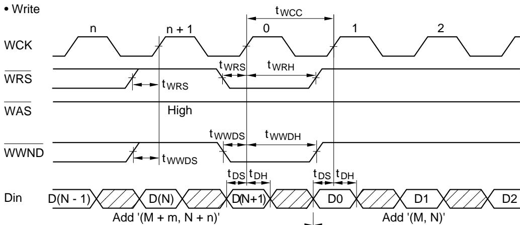
Note: The write address pointer is reset to the window origin address (M, N).
