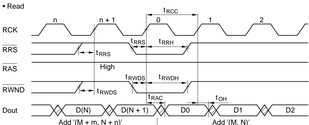
Note: The read address pointer is reset to the window origin address (M, N).
