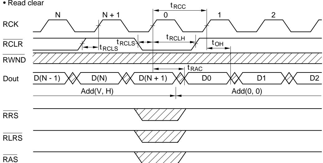
Note: The read address pointer is reset to (0, 0), and window mode is turned off if it was on.
