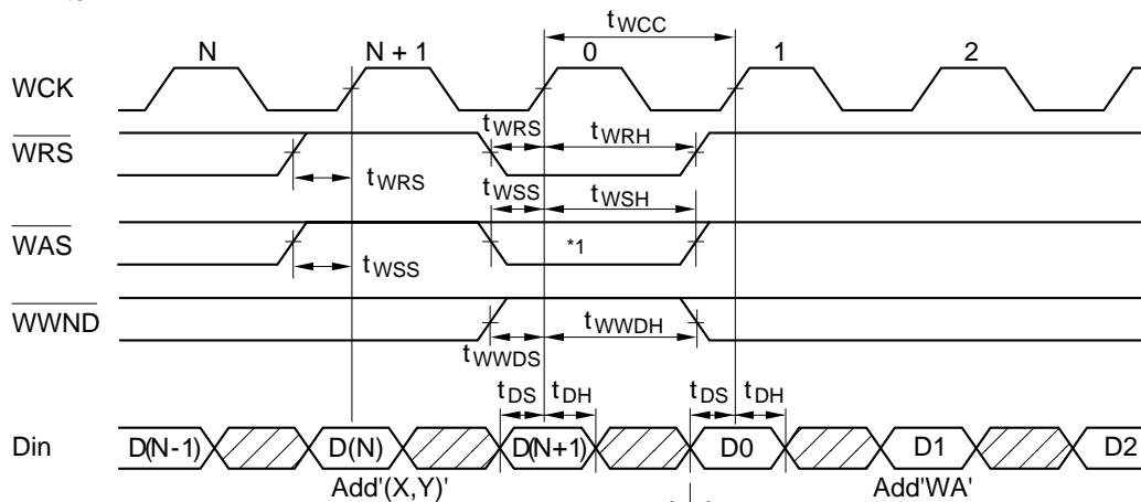
Note: 1. The write address is reset to (0, 0) when WAS is high.
