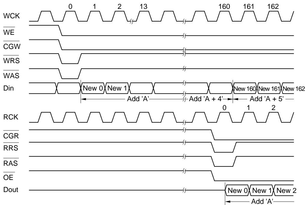
**Note:** Written data can be read out 160 WCK clock cycles after it was written. However, it is necessary to execute the read jump address setup operation outside the time period between 32 WCK cycles before the start of write to that address and 32 WCK cycles after the completion of write to that address.
