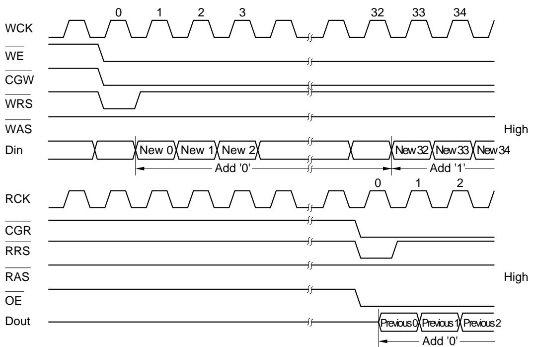
Note: Previous data can be read out up to 32 WCK clock cycles after the write operation.
