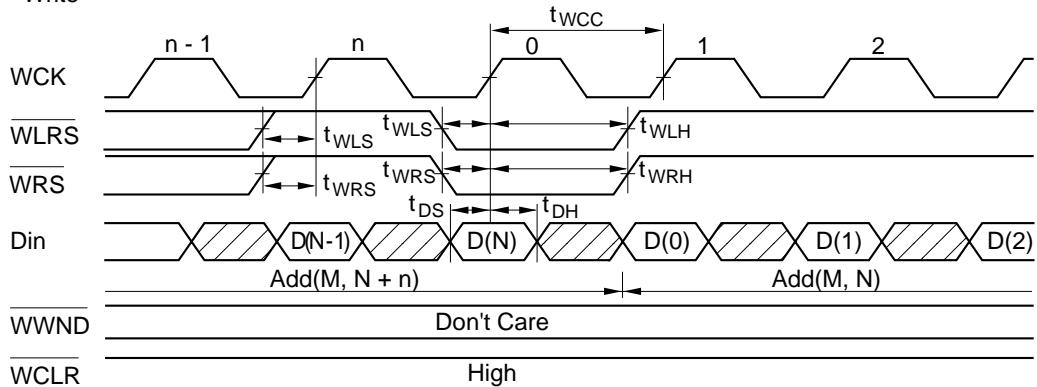
Note: The line address M is held at its current value and the horizontal address currently at  $N + n$  is reset to N.
