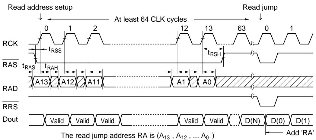
Note: After 64 cycles have passed following the start of read address setup, a jump to the set address can be performed at any time.
