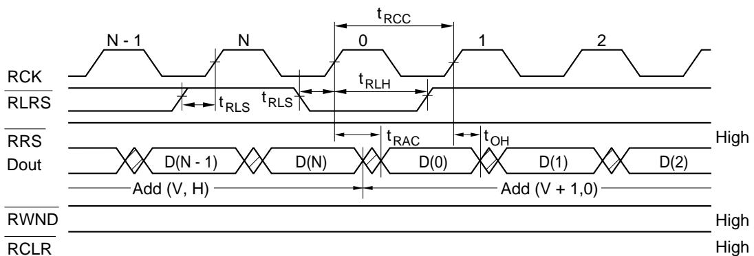
Note: The line address V is incremented, and the horizontal address H is reset to 0.
