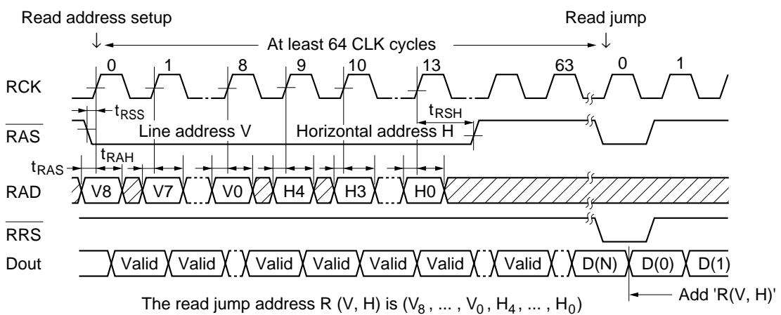
Note: The jump to the set address can be performed at any time once the required 64 cycles have passed following the start of read address setup.
