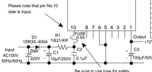
Please verify operation and characteristics in the customer's circuit before actual usage and ensure that the load current does not exceed 0.1A.
