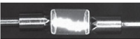
Standard Capacitor with Surface Arc-over
