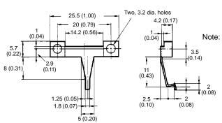
Note: Use the EE1003A Connector Holder to prevent the EE-1003 Connector disconnecting accidentally from the EE-SPZ-A Photomicrosensor.
