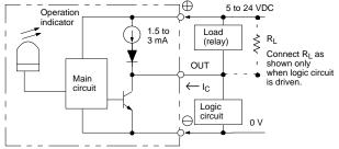
Connect a diode in parallel to the load when an inductive load is connected between + and OUT.
