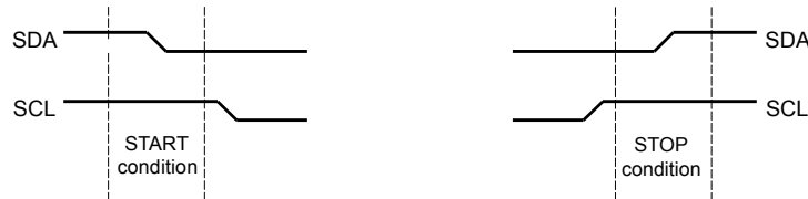
Figure 15-3. START and STOP Conditions
