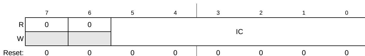
Figure 24-3. I 2 C Frequency Divider Register (I2FDR)
