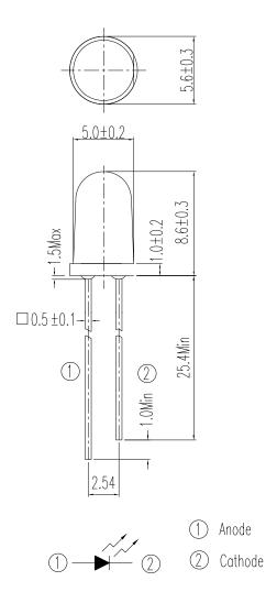
Note: Tolerances unless dimensions ±0.25mm
