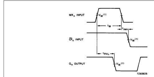
(1) HC :  $V_M$  = 50%;  $V_I$  = GND to  $V_{CC}$ . HCT:  $V_M$  = 1.3 V;  $V_I$  = GND to 3 V.
