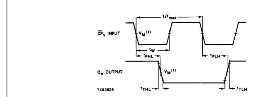
(1) HC :  $V_M$  = 50%;  $V_I$  = GND to  $V_{CC}$ . HCT:  $V_M$  = 1.3 V;  $V_I$  = GND to 3 V.
