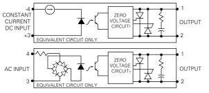
+ Random Turn-on Units have a Random Turn-on circuit instead of Zero Voltage Circuit
