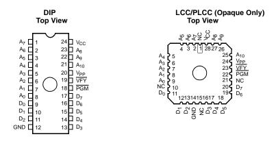
**Figure 1. Programming Pinouts**
