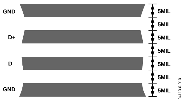
Figure 24. Typical Arrangement of Signal Tracks
