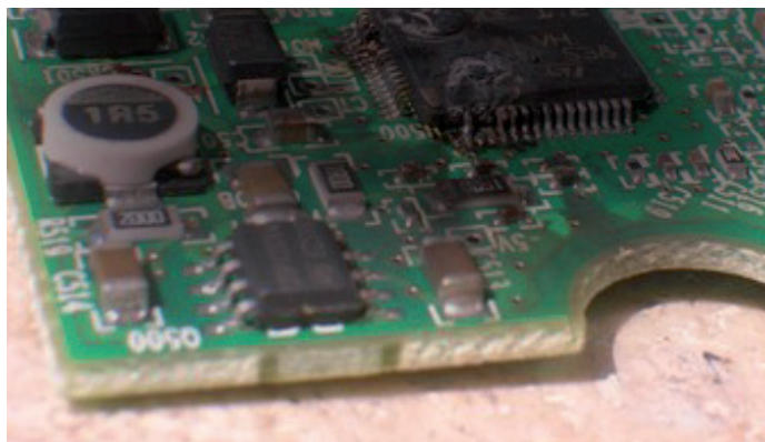
Transient overvoltage effect
