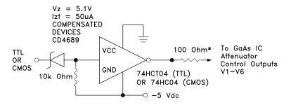
Simple driver using inexpensive standard logic ICs provides fast switching using minimum DC current. \* Recommended value to suppress unwanted RF signals at V1 - V6 control lines.
