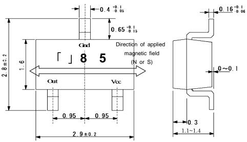
Coplanarity: less than 0.1mm(includiong under reflow condition)
