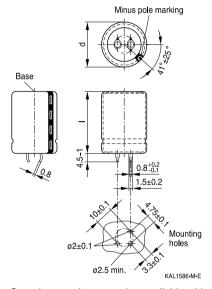
Snap-in capacitors are also available with 3 terminals (length (4.5-1) mm). Safety vent on the base.
