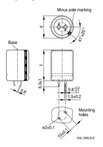
Snap-in terminals, length  $(6.3 \pm 1)$  mm. Also available in a shorter version with a length of (4.5 - 1) mm. Safety vent on the base.
