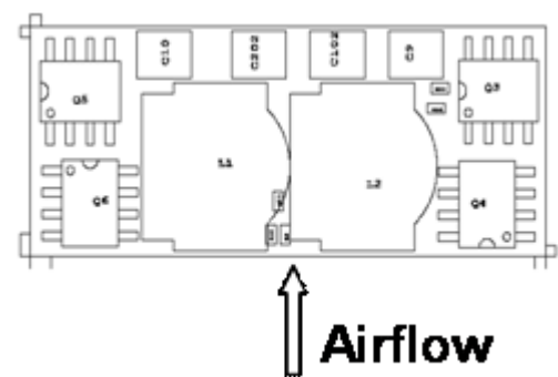
Figure 55. Airflow direction for thermal testing.
