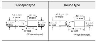
Note: Use crimp terminals having insulation sleeves Recommended crimp terminal: Nominal size 1.25-3
