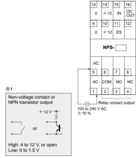
Note: Response time of the NPN open-collector transistor output of NPS-C7 and **NPS-CT7** is 5  $\mu$ s. If a relay or a micro-switch (mechanical contact) is connected, its bounce may result in output chattering. Take care of this aspect, especially when the timer function is used.
