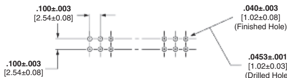
Recommended PC Board Hole Layout (for .055 [1.40] min. thick PC board)
