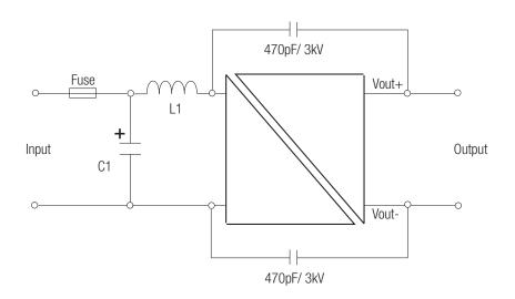
Vin=24V: C1=6.8 $\mu$ F/50V 1812 MLCC, L1 = 10 $\mu$ H, 1.4A, 100m0hm, 0504 SMD Vin=48V: C1= 2.2 $\mu$ F/100V 1812 MLCC, L1 = 10 $\mu$ H, 1.4A, 100m0hm, 0504 SMD
