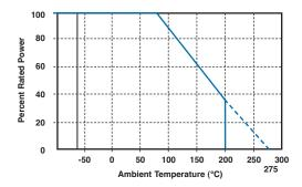
For resistors operated in ambient temperatures above 70°C, power rating must be derated in accordance with this curve.
