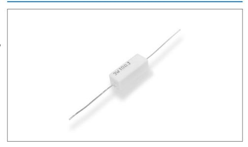
There are some similarities between resistors and fuses in material and structure. Fusible Resistors contain both functions, as a resistor in normal conditions and as a fuse when abnormal currents are applied, so to protect machinery and equipment. Cost savings are apparent as one component is eliminated. The FSQ Fusible Resistor series are produced with precision techniques, enabling precise and stable fusing times.
