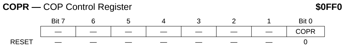
Figure 5-1. COP Control Register
