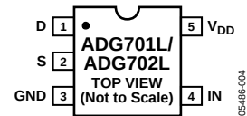
Figure 5. 5-Lead SOT-23 Pin Configuration
