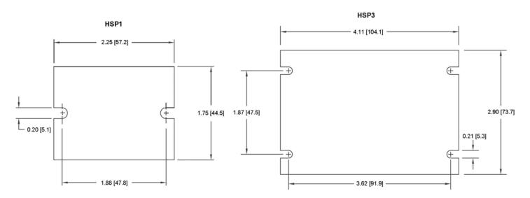
(1) Protective film must be removed from the pad prior to installation of SSR onto heatsink. Failure to remove film may result in relay failure.
