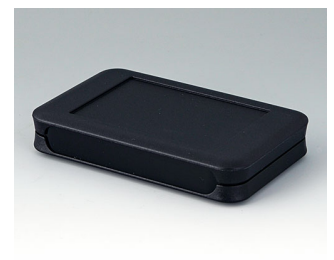
A9051209 SOFT-CASE M PMMA (IR) (UL 94 HB) black RAL 9005 2.56"x4.13"x0.75" IP 54 opt., IP 40
