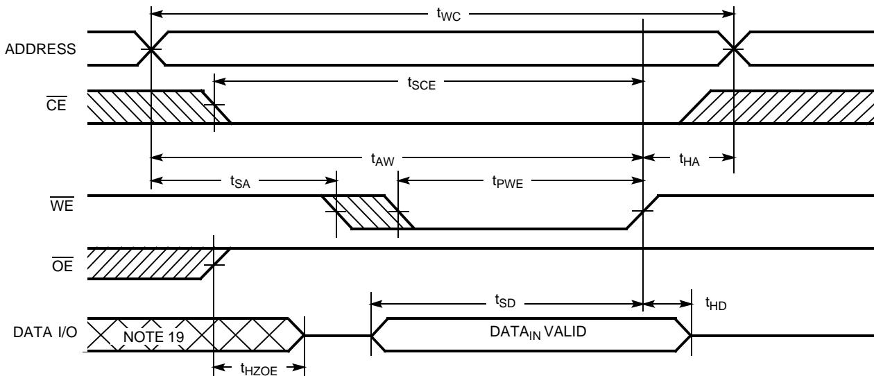
**Write Cycle No. 3 ( $\overline{WE}$  Controlled,  $\overline{OE}$  LOW)<sup>[14, 18]</sup>**
