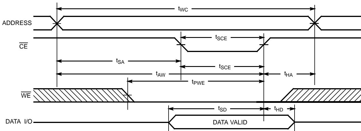
**Write Cycle No. 2 ( $\overline{WE}$  Controlled,  $\overline{OE}$  HIGH During Write)<sup>[14, 17, 18]</sup>**
