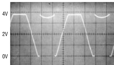
LM324, LM358, OP-20 EXHIBIT OUTPUT PHASE REVERSAL
