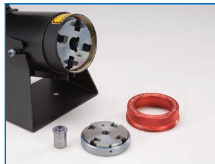
3. Pull out the Locator by hand.
