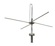
1-port omni ground plane antenna, 30–50 MHz, 360° HPBW, fixed electrical tilt. Bandwidth: 2% of frequency.
