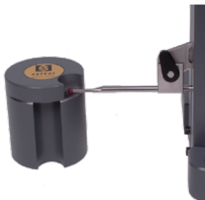
Taking the probe constant value with the setting gage 54-930-202
