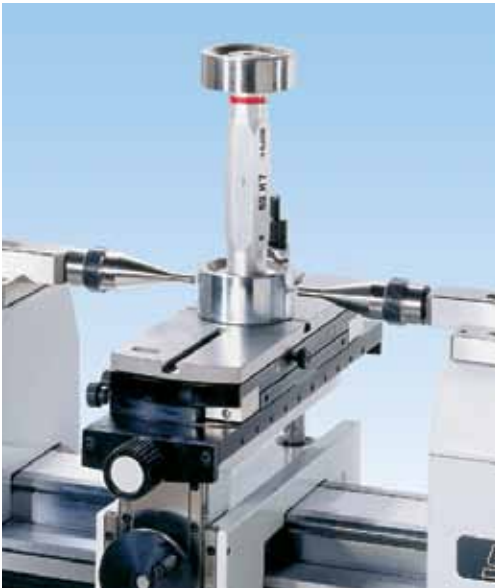
▲ Checking of plug gages and threaded plug gages from dia. 1.18" to 10"/30 to 250mm using table (54-197-011), clamps (54-197-142), small Ø anvils (54-190-806) & thread wires (54-197-007)
