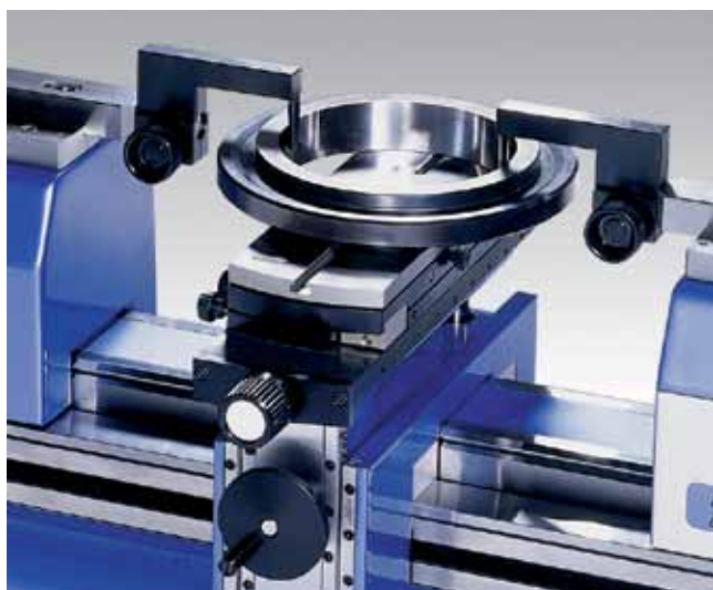
▲ Checking of ring gages from .473 to 10" (12 to 250mm) using table (54-196-160), L-probes (54-197-162) and clamps (54-197-142)
