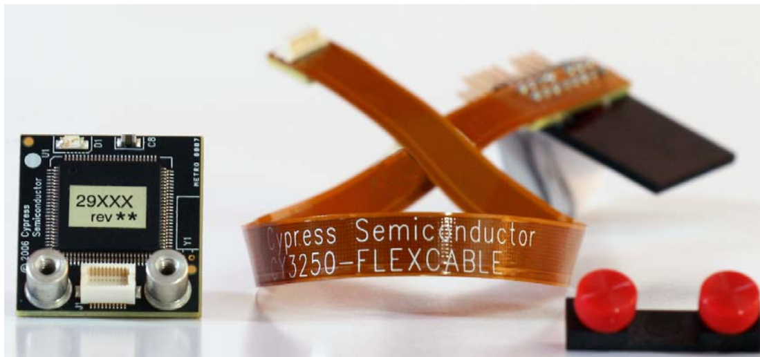
Figure 3-5. Flex Cable and 29000-28 DIP
