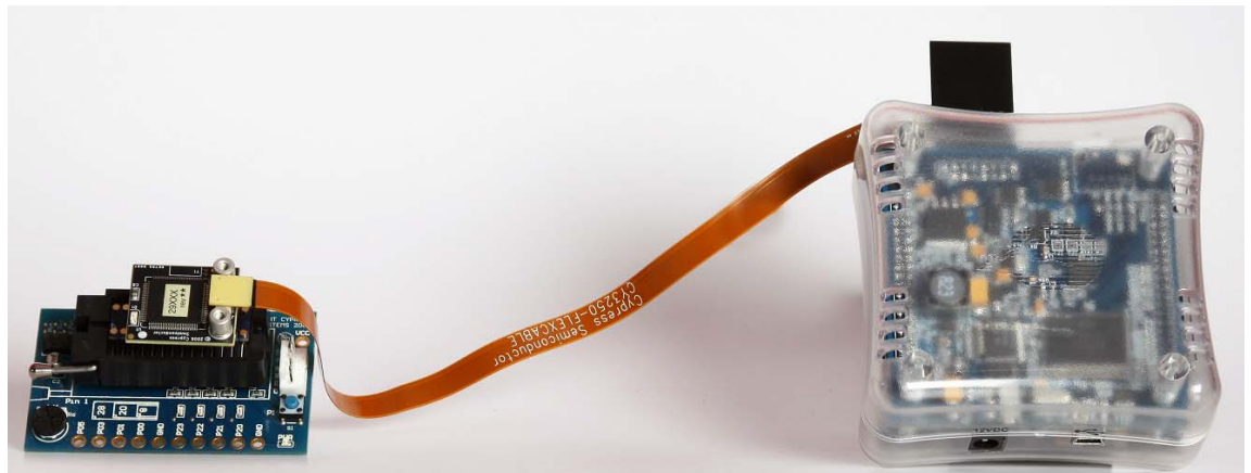
Figure 3-9. Flex Pod Connected to ICE-Cube Pod
