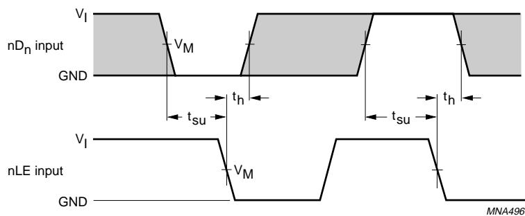
$V_M = 1.5 \text{ V at } V_{CC} \geq 2.7 \text{ V};$  $V_M = 0.5 \times V_{CC} \text{ at } V_{CC} < 2.7 \text{ V}.$ Fig.6 Set-up and hold times for inputs (nD<sub>n</sub>) to inputs (nLE).
