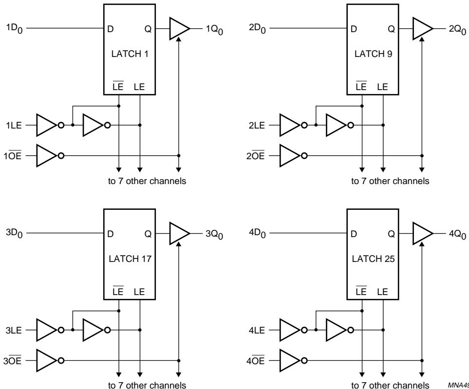
32-bit transparent D-type latch with 5 V tolerant inputs/outputs; 3-state
