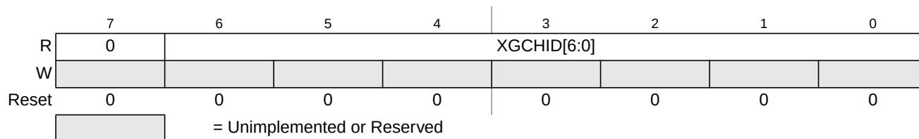
Figure 5-4. XGATE Channel ID Register (XGCHID)
