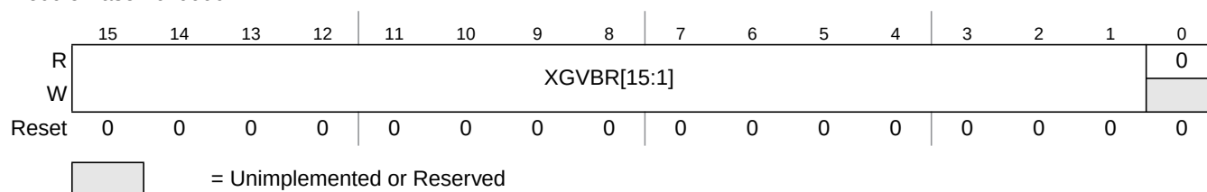
Figure 5-5. XGATE Vector Base Address Register (XGVBR)
