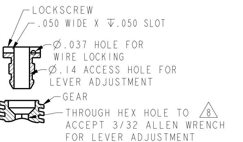
LEVER MAY BE ADJUSTED FOR AN INFINITE NUMBER OF POSITIONS THRU 360°. ADJUSTMENT IS MADE BY LOOSENING THE LOCKING NUT AND THEN THE LOCKSCREW AND TURNING GEAR UNTIL LEVER IS IN DESIRED POSITION. LOCKSCREW AND LOCKNUT ON SHAFT IS THEN TIGHTENED TO POSITIVELY LOCK LEVER IN POSITION.
