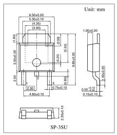
Note) The package of this product will be changed to lead-free type (SP-3SUA). See the new package dimensions section later of this datasheet.
