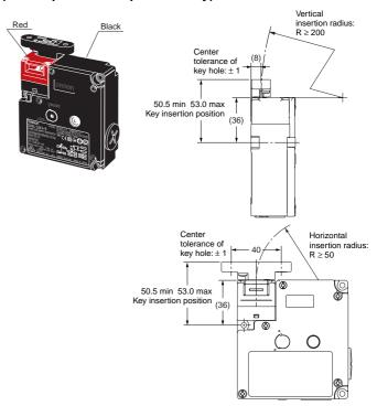
D4NL + D4DS-K5 (with Front-inserted Operation Key)
