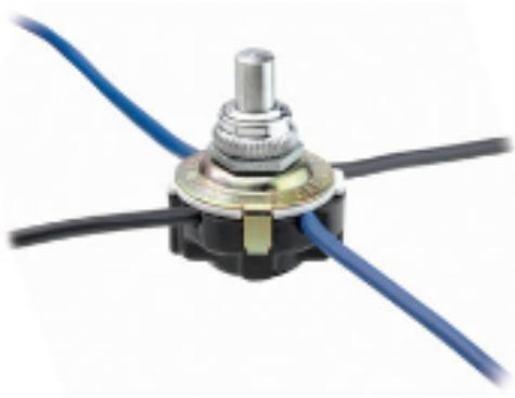
40W-125V AC circuit control, fluorescent starter push button switch, with-nickel push button knob, knurl nut and bushing; 3/8-27 BY 11/32 inch long round male bushing, hex nut. Cover stamped UL/CSA. Knurl nut assembled. Four 6 inch leads, 18awg AWM/TEW 105c 600v plastic, two black and two blue leads, free ends stripped 3/4 inch.
