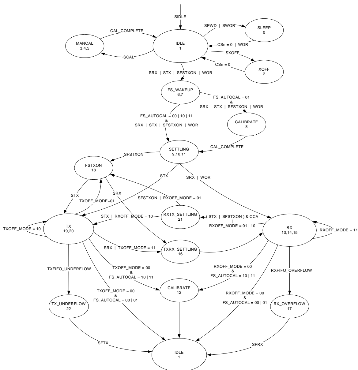
Figure 20: Complete Radio Control State Diagram
