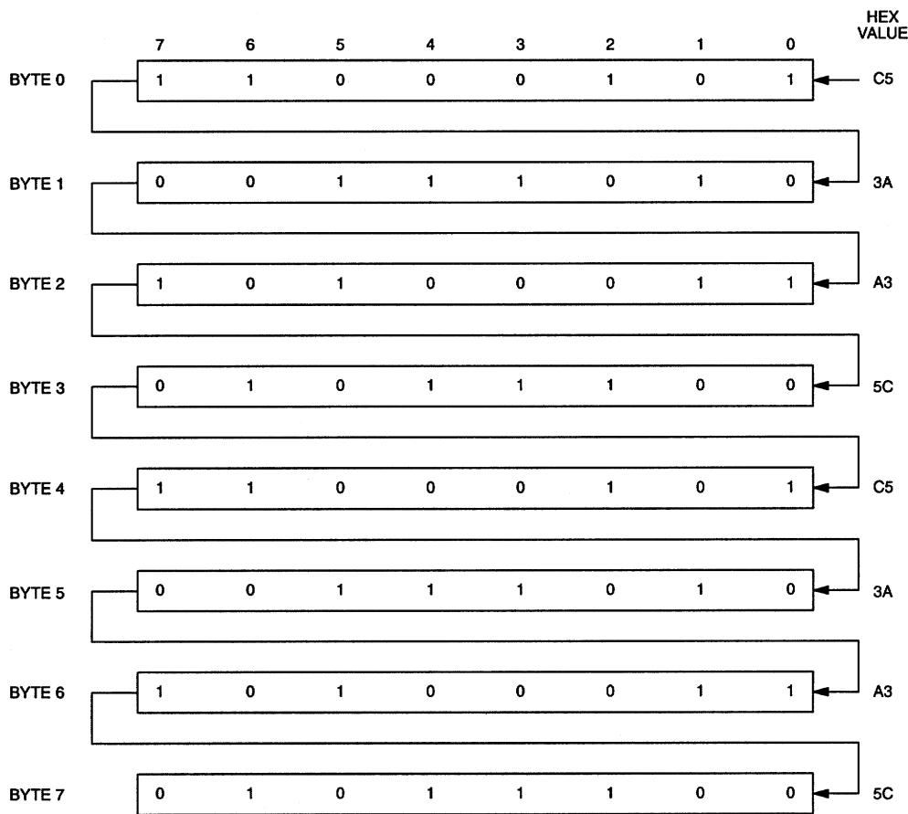
**NOTE:** THE PATTERN RECOGNITION IN HEX IS C5, 3A, A3, 5C, C5, 3A, A3, 5C. THE ODDS OF THIS PATTERN BEING ACCIDENTALLY DUPLICATED AND CAUSING INADVERTENT ENTRY TO THE PHANTOM CLOCK IS LESS THAN 1 IN  $10^{19}$ . THIS PATTERN IS SENT TO THE PHANTOM CLOCK LSB TO MSB.
