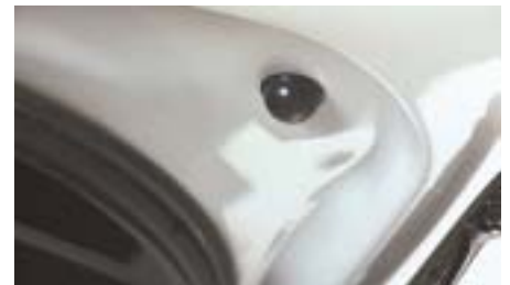
Rear Windshield Sound Dampers Fig.102
